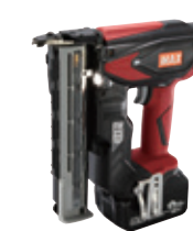
Our “battery-operated finishing nailer for frames” whose emphasis has been placed on efficiency in fixing work for forms.
