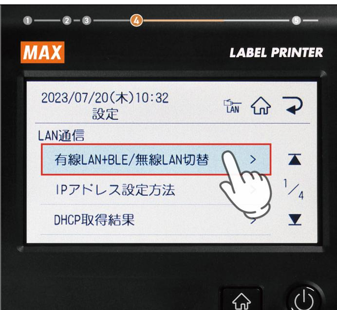
The image shows the MAX LABEL PRINTER LAN switching screen. At the top, there is a progress bar with steps 1 through 5, and step 4 is highlighted. The screen displays the date and time '2023/07/20(木)10:32' and the title '設定'. Below the title is the section 'LAN通信'. There are three menu items: '有線LAN+BLE/無線LAN切替', 'IPアドレス設定方法', and 'DHCP取得結果'. The '有線LAN+BLE/無線LAN切替' item is highlighted with a red box and a hand cursor pointing to it.
