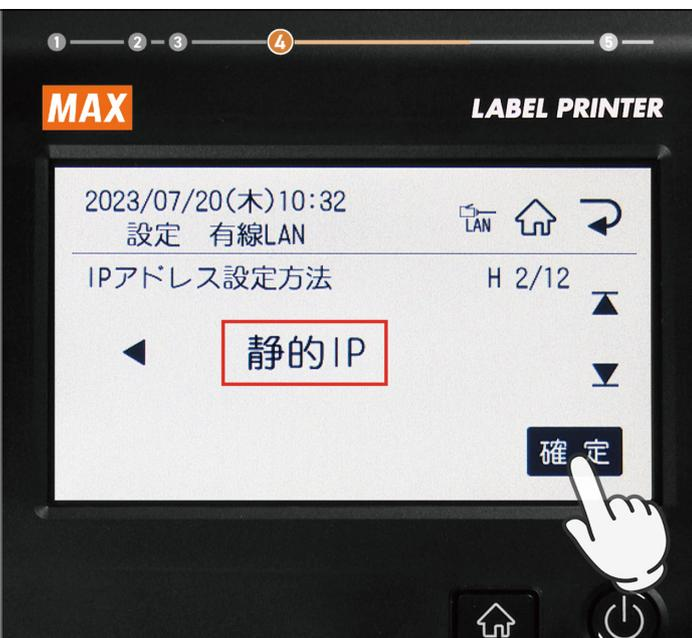
The image shows the MAX LABEL PRINTER's touch screen interface. The progress bar is at step 4 of 5. The screen displays '2023/07/20(木)10:32' and '設定 有線LAN'. Below the LAN, home, and back icons, the title is 'IPアドレス設定方法'. The menu shows '静的IP' with a left arrow and 'H 2/12' on the right. The option '静的IP' is highlighted with a red box. A hand icon is shown pointing to the '確定' (Confirm) button at the bottom right.
