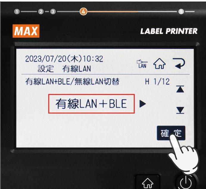
The image shows the MAX LABEL PRINTER's touch screen interface. At the top, a progress bar indicates step 4 of 5. The screen displays the date and time '2023/07/20(木)10:32' and the title '設定 有線LAN'. Below this, there are icons for LAN, home, and back. The main menu shows '有線LAN+BLE/無線LAN切替' with 'H 1/12' on the right. The option '有線LAN+BLE' is highlighted with a red box. A hand icon is shown pointing to the '確定' (Confirm) button at the bottom right.
